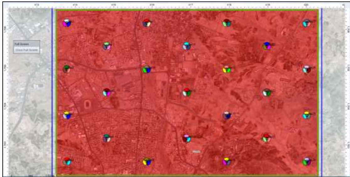
Figure 4. 80: prediction result of Effective Service Area Analysis (DL+UL) in 5G NR technology (Before optimization)
