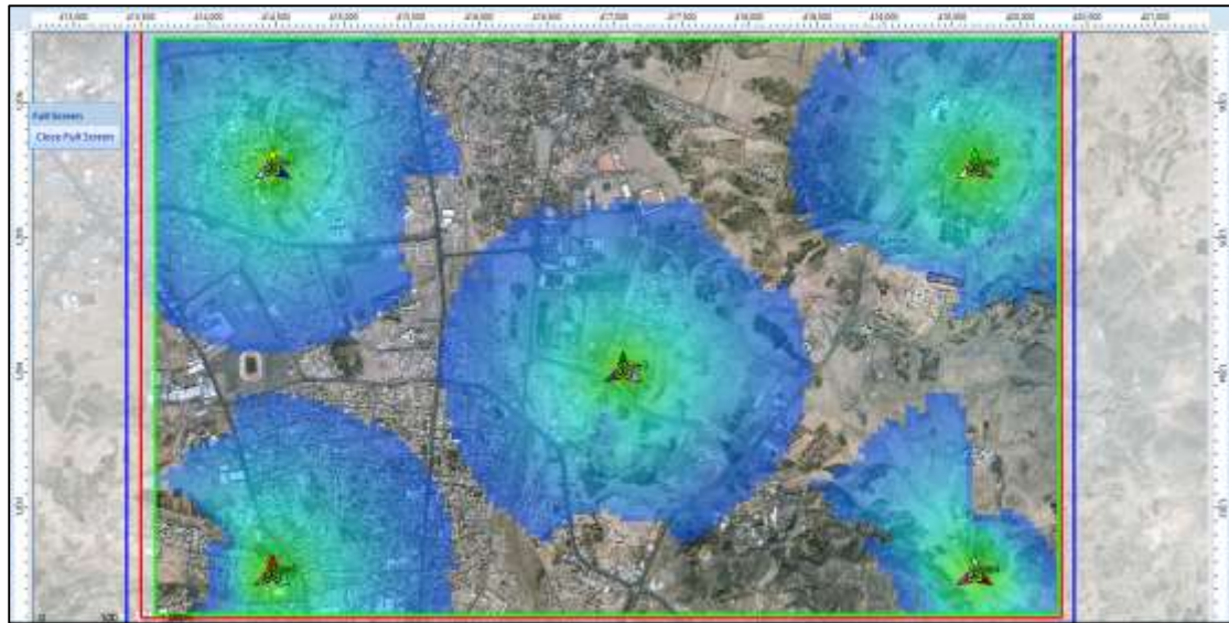
Figure 4.11: prediction result of Effective Signal Analysis (DL) in LTE technology (Before optimization)
