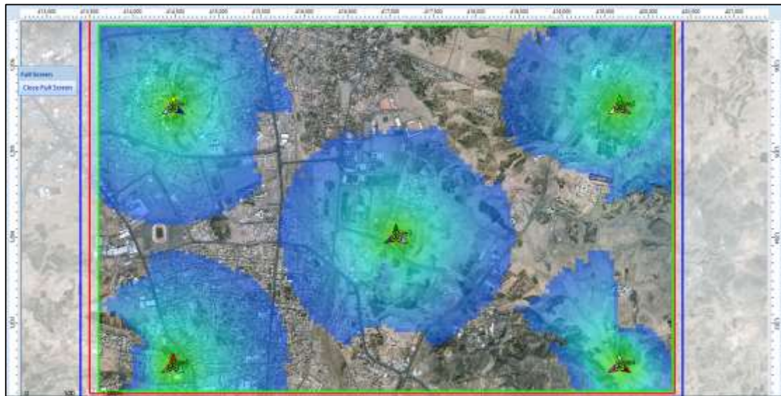
Figure 3. 33: prediction result of Effective Signal Analysis (DL) in LTE technology
