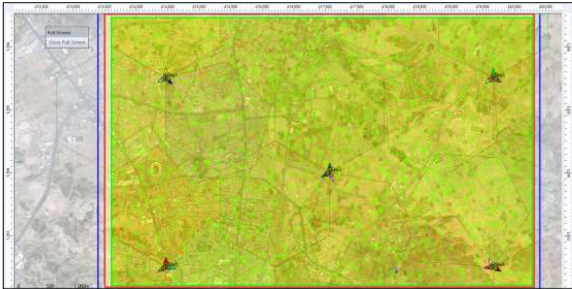
Figure 4. 24: prediction result of Coverage by C/(I+N) Level (UL) in LTE technology (After optimization)
