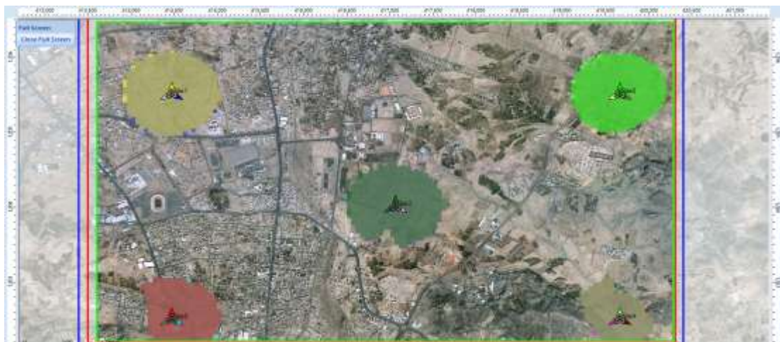
Figure 3. 28: prediction result of Coverage by Transmitter (DL) in LTE technology
