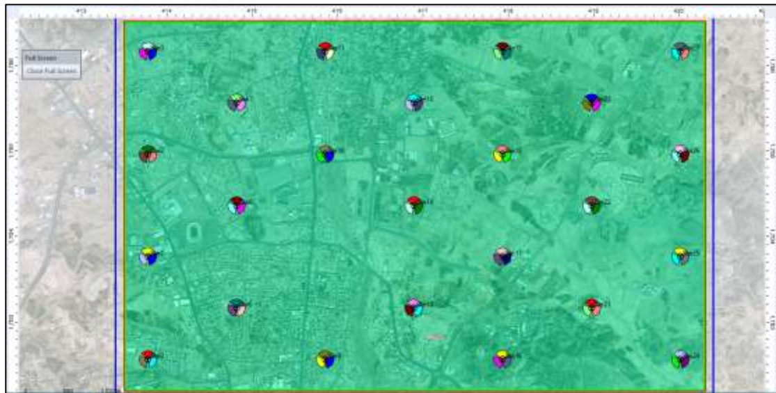
Figure 3. 64: prediction result of 5G NR: Uplink Service Areas in 5G NR technology
