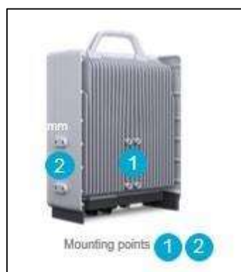
Figure 2. 23: Remote Radio Head
