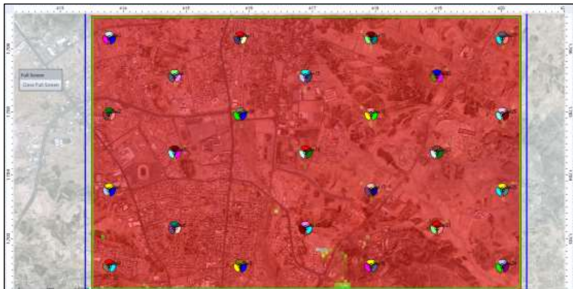
Figure 4. 60: prediction result of 5G NR: Downlink Capacity in 5G NR technology (Before optimization)
