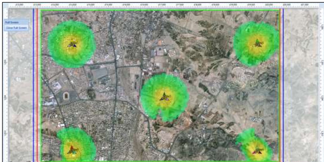
Figure 4. 23: prediction result of Coverage by C/(I+N) Level (UL) in LTE technology (Before optimization)
