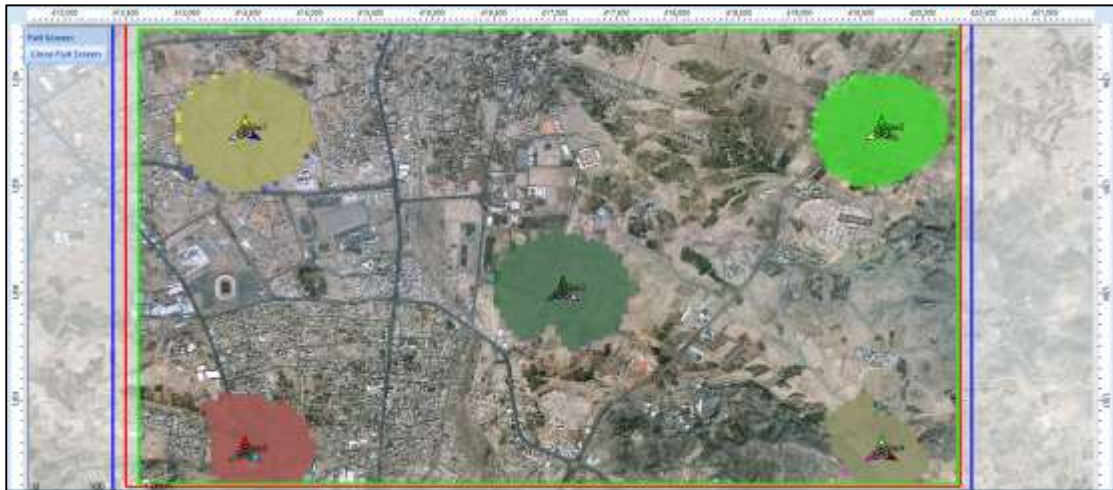
Figure 4. 3: prediction result of Coverage by Signal Level (DL) in LTE technology (Before optimization)
