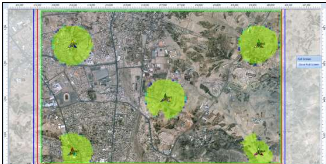
Figure 4. 7: prediction histogram of Coverage by Signal Level (DL) in LTE technology (Before optimization)
