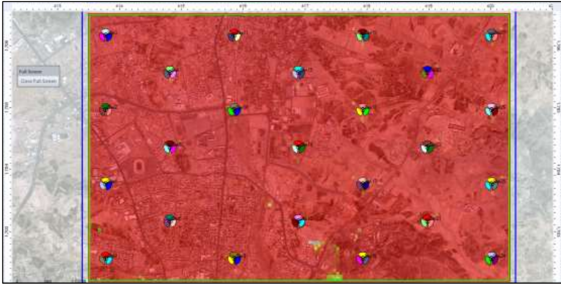
Figure 4. 61: prediction result of 5G NR: Downlink Capacity in 5G NR technology (After optimization)
