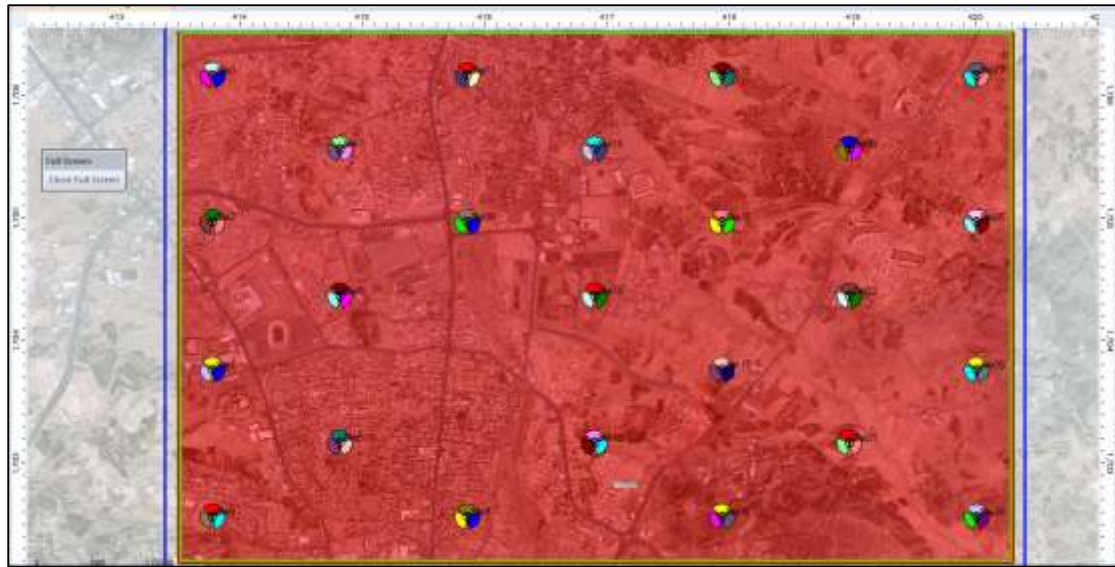
Figure 3. 69: prediction result of Coverage by Throughput (DL) in 5G NR technology
