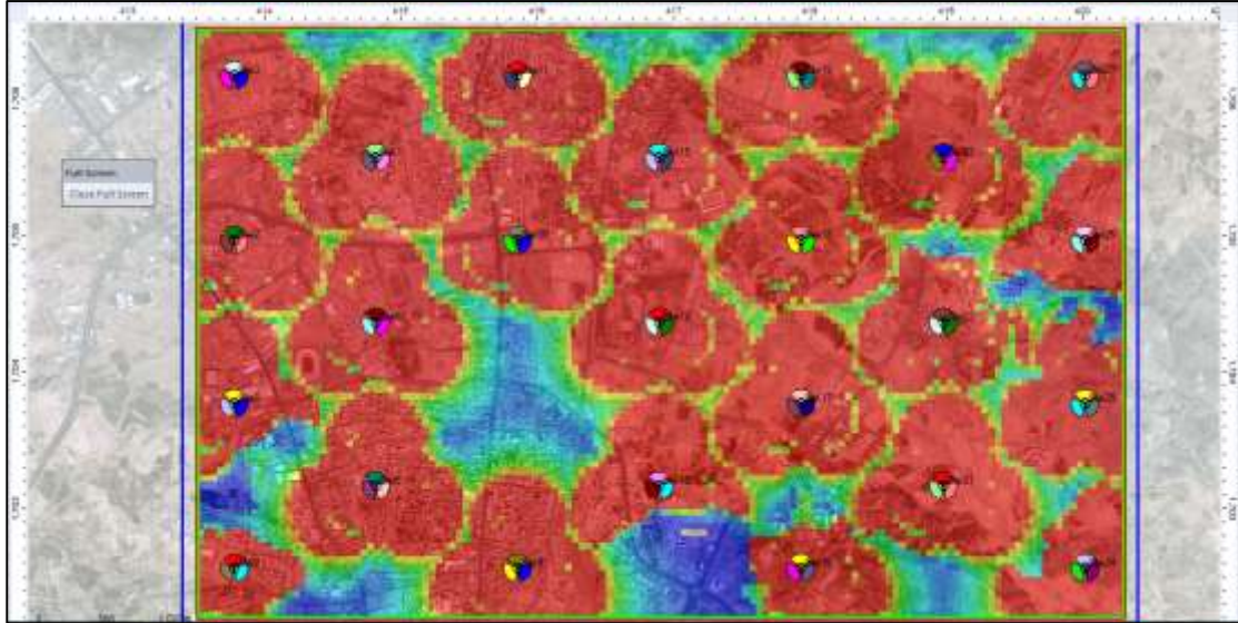
Figure 3. 66: prediction result of 5G NR: Uplink Capacity in 5G NR technology
